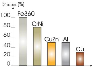
**Fig. 5** The rated operating distance is reduced by the use of metals and alloys other than Fe360. The most important reduction factors for inductive proximity sensors are shown in the figure.
