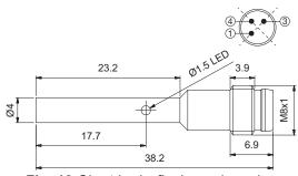
Fig. 12 Short body, flush version, plug
