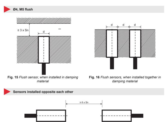
**Fig. 17** For sensors installed opposite each other, a minimum space of 6 x Sn (the nominal sensing distance) must be observed
