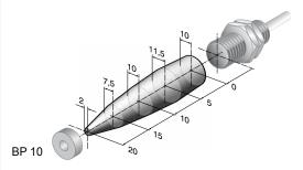
s<sub>ao</sub> = 20 mm (BP 10, BP 15 SS) assured switching distance:
