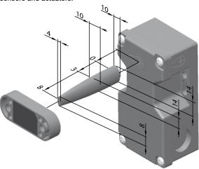
$s_{ao}$  = 8 mm Assured switching distance:  $s_{ar} = 18 \text{ mm}$ Assured switch-off distance:
