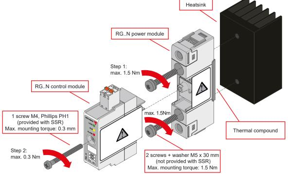
Step 1: Mount RG..N power module to Heatsink
