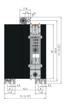
Housing width tolerance +0.5mm, -0mm as per DIN 43880.
