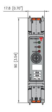
Housing width tolerance +0.5mm, -0mm as per DIN 43880. All other tolerances +/- 0.5mm. Dimensions in mm.
